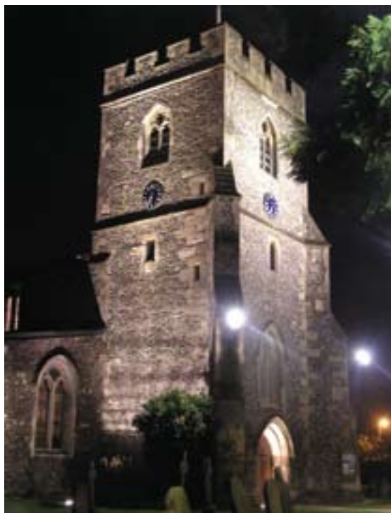
The tower floodlights are run via a solar clock which turns them on at dusk and off again at a set time.
