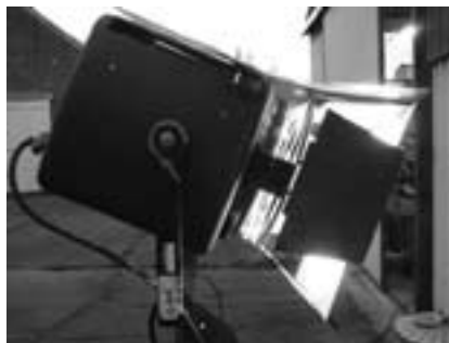
Vertical projection angle (top) creates distortion of the image (below).
