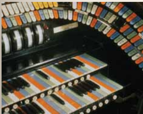
Light Console detail, London Coliseum 1952, 216 dimmers.
